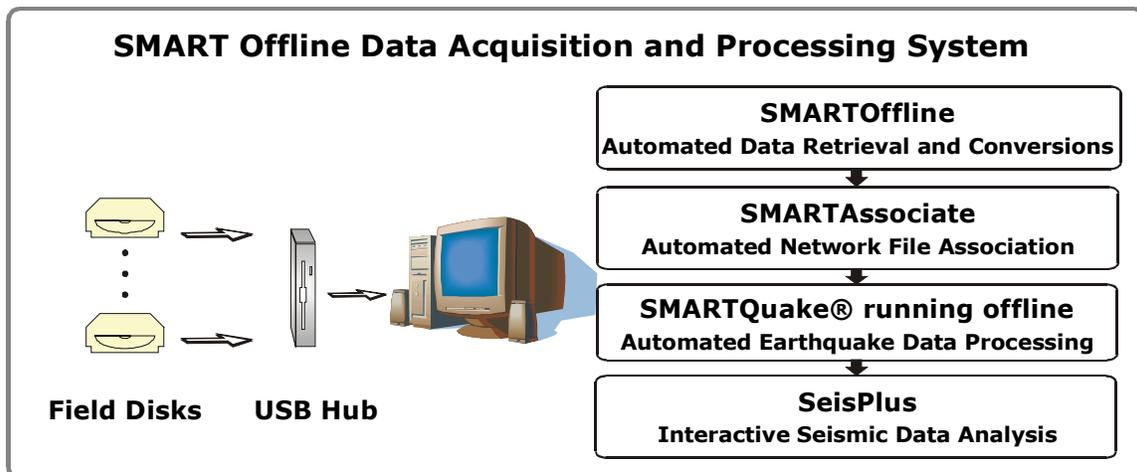
Figure 9. SMART Offline Data Acquisition and Processing
